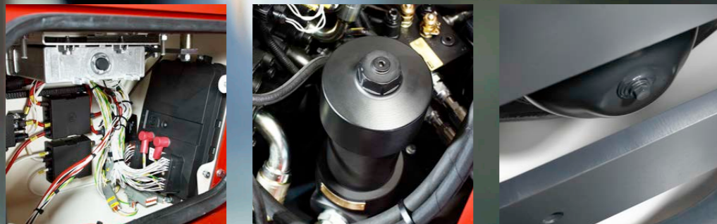
Service is fast, simple and convenient thanks to improved accessibility and smart features, like the hydraulic filters (middle) and a plug for filling shaft oil while standing (right).
